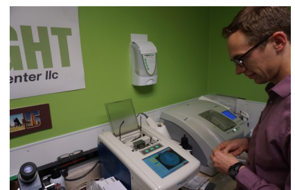
Dr. DeMeritt cutting a prescription lens to fit a frame
